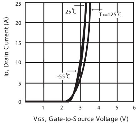
Figure 2. Transfer Characteristics
