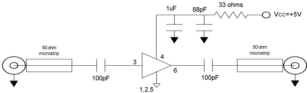
**Application Schematic for +5V Operation at 1900 MHz**
