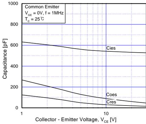
**Fig 7. Capacitance Characteristics**
