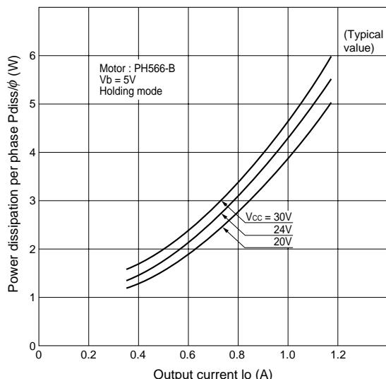
Fig. D SI-7500A Derating curve
