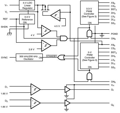
FIGURE 2. Si786 Block Diagram
