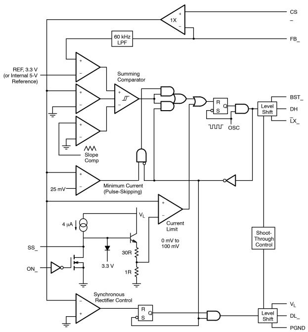
FIGURE 3. Si786 Controller Block Diagram
