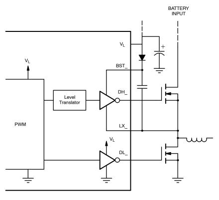
FIGURE 4. Boost Supply for Gate Drivers
