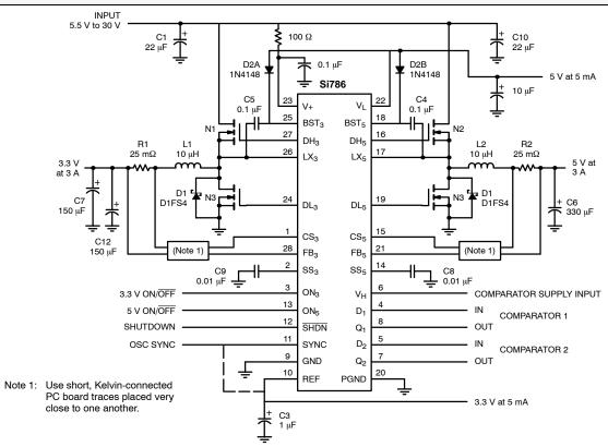
FIGURE 1. Si786 Application Circuit
