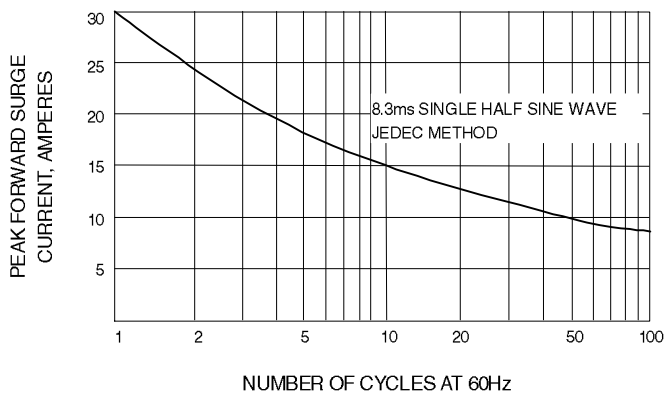
Fig. 3-MAXIMUM NON-REPETITIVE SURGE CURRENT
