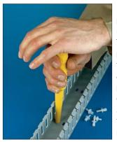
HellermannTyton panel rivets are one piece drive rivets that provide a fast, economical means of affixing wiring duct. The rivet is inserted into a 3/16" prepunched hole and the pin is driven into the base, thereby expanding the rivet legs and locking the duct and sub-panel in place. The panel thickness (including the duct thickness) should be a maximum of 3/16". A panel rivet tool is also available for quick and easy installation of the drive rivets.
