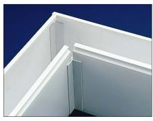
HellermannTyton corner strips are supplied in six foot lengths which can be cut to provide a rounded corner for two duct sections meeting at right angles. They are made from PVC material and can be used with any size HellermannTyton wiring duct.
