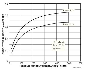
FIGURE 5A. HOLD-CURRENT RESISTANCE (SLA7024M and SMA7029M)
