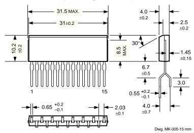
NOTE: Exact body and lead configuration at vendor's option within limits shown.
