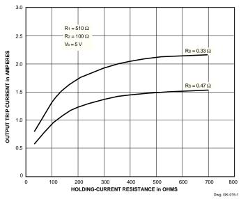
FIGURE 5B. HOLD-CURRENT RESISTANCE (SLA7026M)
