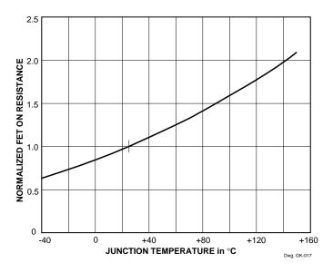
FIGURE 8. NORMALIZED ON RESISTANCE vs TEMPERATURE
