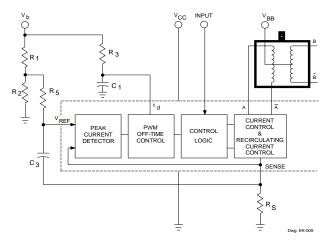
FIGURE 2. PWM CONTROL (RUN MODE)
