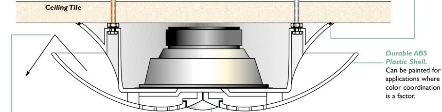
Wide Dispersion of Sound. A combination of direct and reflected sound paths produce a clear, wide dispersion of high-quality sound, even at higher frequencies where other speakers begin to beam. This enhances intelligibility and makes exact speaker placement less critical.
