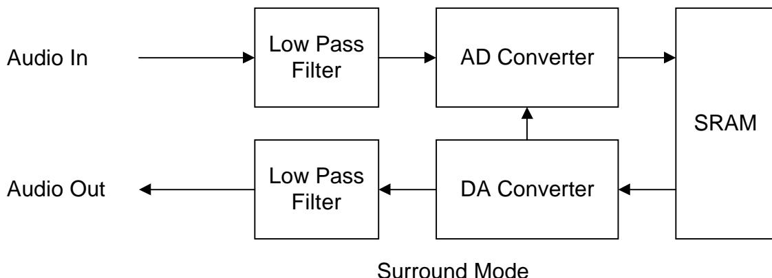
When EC/SR pin is tie to VDD then SM7183 is set to Echo Mode. When EC/SR pin is tie to GND then SM7183 is set to Surround Mode. The only difference between echo mode and surround mode are there is no feed back & add path inside the SM7183. And the delay time is shorter for surround mode then echo mode. But surround mode provide higher sampling rate and better sound quality then echo mode.
