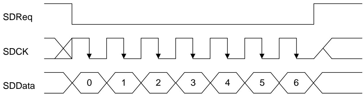
When SDREQ is low then SM7183 is ready for received data from SDDATA. SM7183 will latch the SDDATA using the SDCK's negative edge.
