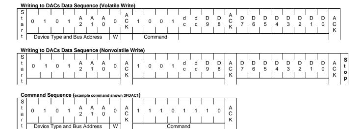
The third example illustrates the data sequence for a two-byte command.
