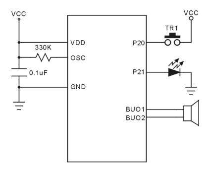
Note: Please bonds all of  $V_{\text{DD}}$  and  $V_{\text{SS}}$  pins.
