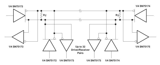
NOTE A: The line should be terminated at both ends in its characteristicc impedance ( $R_T = Z_O$ ). Stub lengths off the main line should be kept as short as possible.
