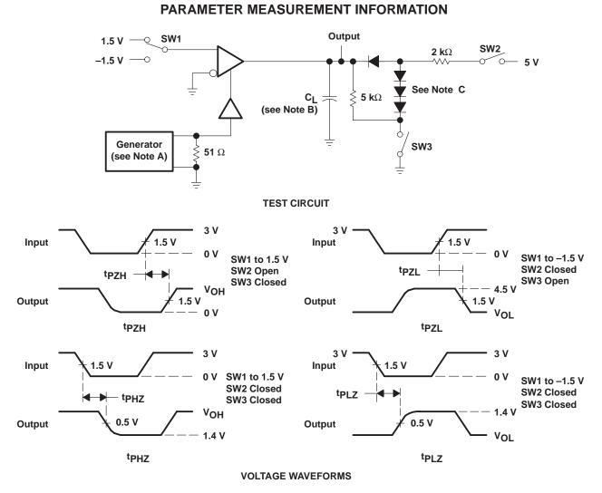
NOTES: A. The input pulse is supplied by a generator having the following characteristics: PRR  $\leq$  1 MHz, duty cycle = 50%, tf  $\leq$  6 ns, t<sub>f</sub>  $\leq$  6 ns, Z<sub>O</sub> = 50  $\Omega$ .
