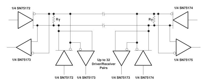
NOTE A: The line should be terminated at both ends in its characteristicc impedance (R<sub>T</sub> = Z<sub>O</sub>). Stub lengths off the main line should be kept as short as possible.
