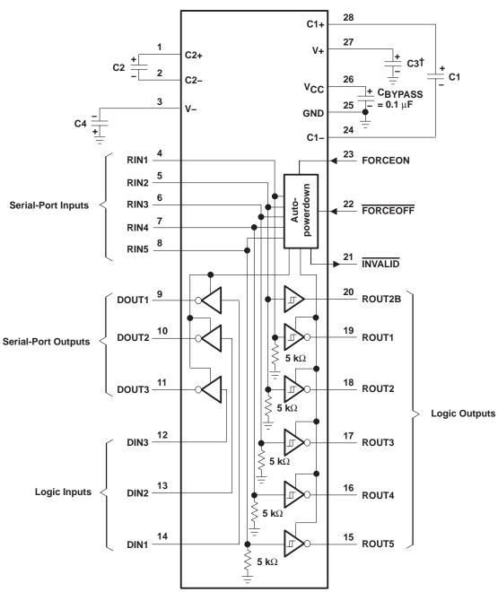
†C3 can be connected to V<sub>CC</sub> or GND. NOTE A: Resistor values shown are nominal.
