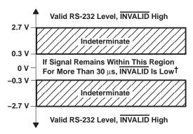
$<sup>^{\</sup>dagger}$ Auto-powerdown disables drivers and reduces supply current to 1  $\mu$ A.
