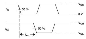
NOTE: All V<sub>I</sub> input pulses are supplied by a generator having the following characteristics: t<sub>r</sub> or t<sub>f</sub> ≤ 6 ns, Pulse Repetition Rate (PRR) = 25 kHz, 50% duty cycle
