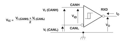
Figure 5. Receiver Voltage and Current Definitions
