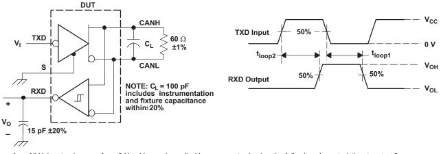
A. All V<sub>1</sub> input pulses are from 0 V to V<sub>CC</sub> and supplied by a generator having the following characteristics:  $t_r$  or  $t_f \le 6$  ns. Pulse Repetition Rate (PRR) = 125 kHz, 50% duty cycle.
