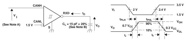
A. The input pulse is supplied by a generator having the following characteristics: PRR  $\leq$  125 kHz, 50% duty cycle, t<sub>f</sub> $\leq$  6 ns, t<sub>f</sub> $\leq$  6 ns, Z<sub>0</sub> = 50  $\Omega$ .
