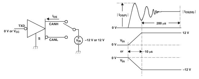
Figure 11. Driver Short-Circuit Current Test and Waveform
