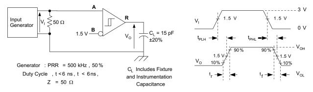
Figure 7. Receiver Switching Test Circuit and Voltage Waveforms
