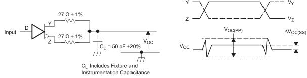
Input: PRR = 500 kHz, 50% Duty Cycle,t  $_r$ <6ns,  $t_f$ <6ns,  $Z_O$  = 50  $\Omega$
