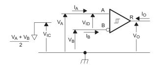
Figure 6. Receiver Voltage and Current Definitions
