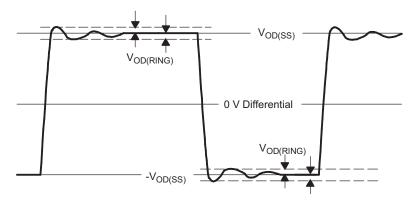
Figure 3. V<sub>OD(RING)</sub> Waveform and Definitions
