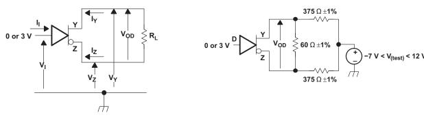
Figure 1. Driver V<sub>OD</sub> Test Circuit: Voltage and Current Definitions
