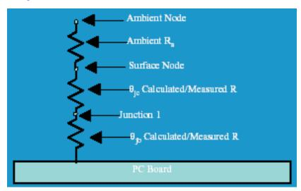
Figure 15. Thermal Resistance
