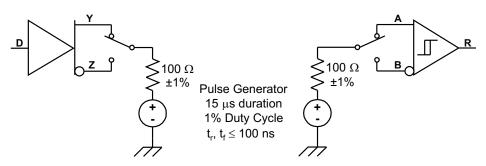
Figure 8. Test Circuit, Transient Overvoltage Test
