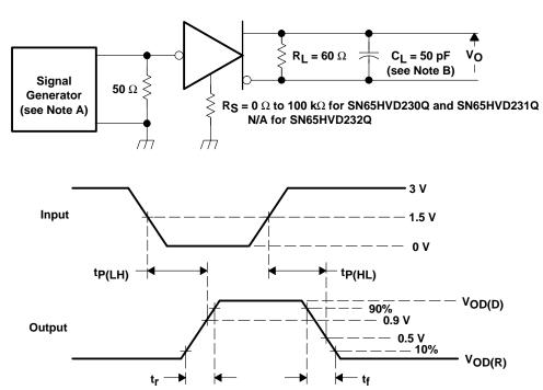
NOTES: A. The input pulse is supplied by a generator having the following characteristics: PRR  $\leq$  500 kHz, 50% duty cycle,  $t_r \leq$  6 ns,  $t_f \leq$  6 ns,  $Z_0 = 50 \Omega$ .
