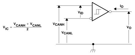
Figure 5. Receiver Voltage and Current Definitions
