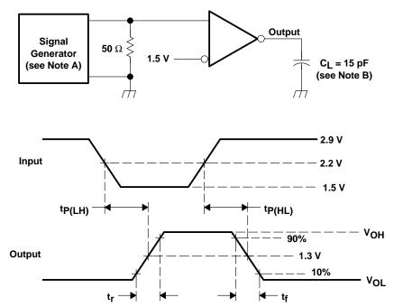
NOTES: A. The input pulse is supplied by a generator having the following characteristics: PRR  $\leq$  500 kHz, 50% duty cycle,  $t_{\Gamma} \leq$  6 ns,  $t_{f} \leq$  7 ns,  $t_{f} \leq$  8 ns,  $t_{f} \leq$  8 ns,  $t_{f} \leq$  9 ns,
