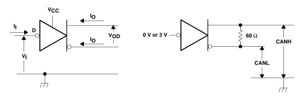
Figure 1. Driver Voltage and Current Definitions
