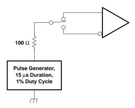
Figure 7. Overvoltage Protection
