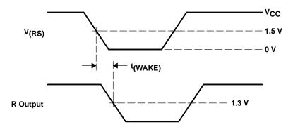
Figure 8. t<sub>(WAKE)</sub> Test Circuit and Voltage Waveforms
