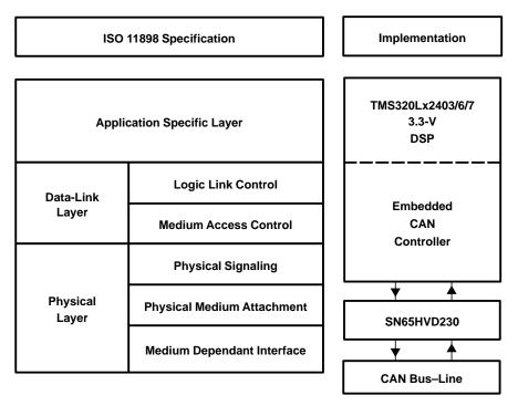
Figure 26. The Layered ISO 11898 Standard Architecture
