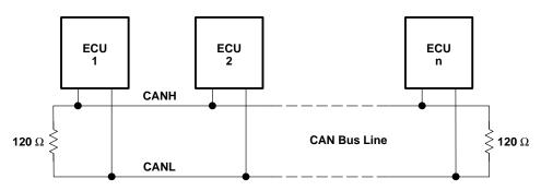
Figure 28. Typical CAN Network
