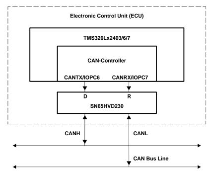
Figure 27. Details of a Typical CAN Node
