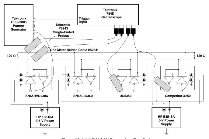
Figure 35. 3.3-V/5-V CAN Transceiver Test Bed
