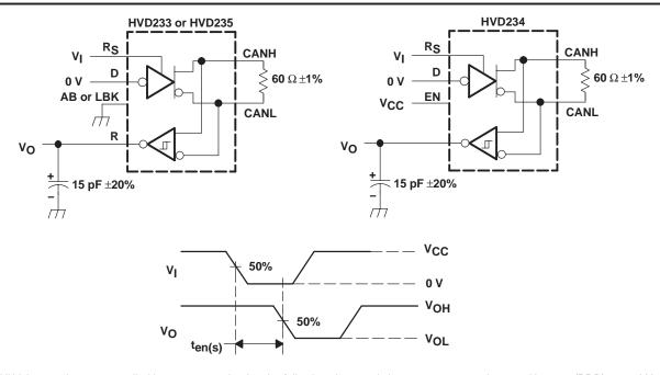
NOTE: All V<sub>I</sub> input pulses are supplied by a generator having the following characteristics: t<sub>r</sub> or t<sub>f</sub> ≤ 6 ns, pulse repetition rate (PRR) = 125 kHz, 50% duty cycle.
