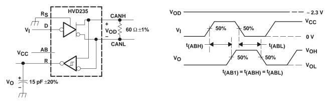
NOTE: All V<sub>I</sub> input pulses are supplied by a generator having the following characteristics:  $t_{\Gamma}$  or  $t_f \le 6$  ns, pulse repetition rate (PRR) = 125 kHz, 50% duty cycle.
