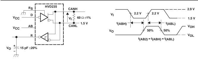
NOTE: All V<sub>I</sub> input pulses are supplied by a generator having the following characteristics:  $t_{\Gamma}$  or  $t_{\Gamma} \le 6$  ns, pulse repetition rate (PRR) = 125 kHz, 50% duty cycle.
