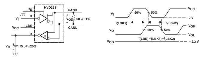
NOTE: All V<sub>I</sub> input pulses are supplied by a generator having the following characteristics:  $t_r$  or  $t_f \le 6$  ns, pulse repetition rate (PRR) = 125 kHz, 50% duty cycle.
