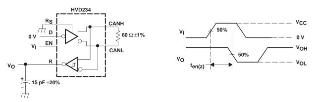
NOTE: All V<sub>I</sub> input pulses are supplied by a generator having the following characteristics:  $t_r$  or  $t_f \le 6$  ns, pulse repetition rate (PRR) = 50 kHz, 50% duty cycle.
