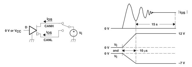
Figure 15. IOS Test Circuit and Waveforms
