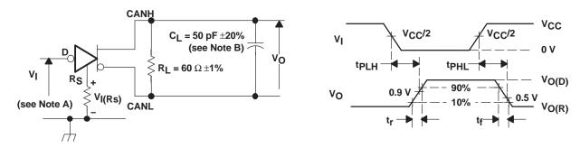
NOTES:A. The input pulse is supplied by a generator having the following characteristics: Pulse repetition rate (PRR)  $\leq$  125 kHz, 50% duty cycle,  $t_f \leq$  6ns,  $t_f \leq$  6ns,  $t_O = 50\Omega$ .
