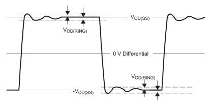
Figure 3.  $V_{OD(RING)}$  Waveform and Definitions
