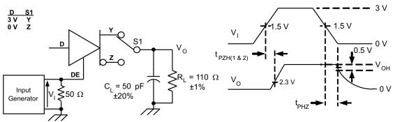
Generator: PRR = 50 kHz, 50% Duty Cycle,  $t_r < 6 \text{ ns}$ ,  $t_f < 6 \text{ ns}$ ,  $Z_0 = 50 \Omega$ C<sub>1</sub> Includes Fixture and Instrumentation Capacitance
