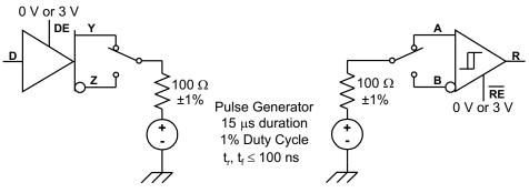
Figure 12. Test Circuit, Transient Over Voltage Test
