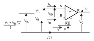
Figure 8. Receiver Voltage and Current Definitions
