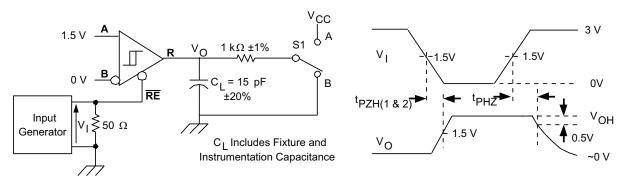
Generator: PRR = 50 kHz, 50% Duty Cycle,  $t_r$  < 6 ns,  $t_f$  < 6 ns,  $Z_0$  = 50  $\Omega$
