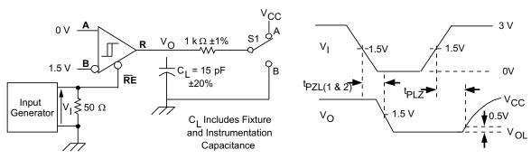
Generator: PRR = 50 kHz, 50% Duty Cycle,  $t_{\rm r}$  < 6 ns,  $t_{\rm f}$  < 6 ns, Z  $_0$  = 50  $~\Omega$
