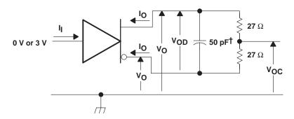
† Includes probe and jig capacitance
