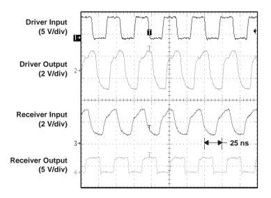
Figure 22. Signal Waveforms at 50 Mbps
