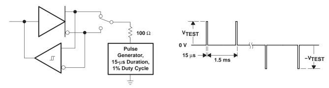
Figure 12. Test Circuit and Waveform, Transient Over Voltage Test
