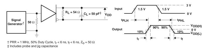
Figure 3. Driver Switching Test Circuit and Waveforms, 485-Loading
