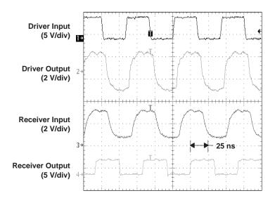
Figure 20. Signal Waveforms at 30 Mbps
