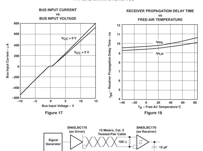
Figure 19. Circuit Diagram for Signaling Characteristics
