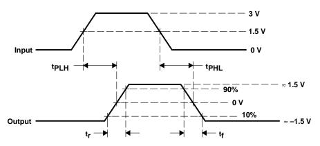
Figure 4. Output Switching Test Circuit and Waveforms
