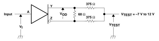
Figure 2. Test Circuit,  $V_{\mbox{OD}}$  With Common-Mode Loading
