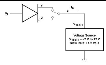
Figure 7. Test Circuit, Short-Circuit Output Current
