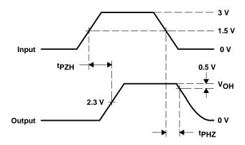
Figure 5. Enable Timing Test Circuit and Waveforms, tPZH and tPHZ
