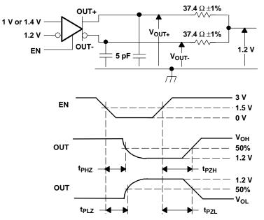
NOTE: All input pulses are supplied by a generator having the following characteristics:  $t_r$  or  $t_f \le 1$  ns, pulse-repetition rate (PRR) = 0.5 Mpps, pulse width = 500 ± 10 ns.  $C_L$  includes instrumentation and fixture capacitance within 0,06 mm of the D.U.T.
