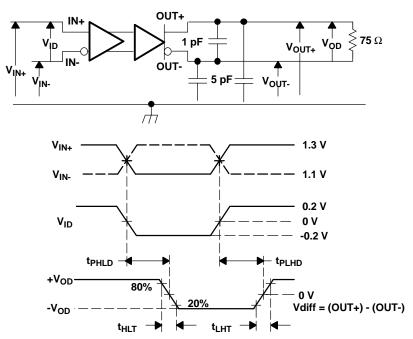
NOTE: All input pulses are supplied by a generator having the following characteristics:  $t_r$  or  $t_f \le .25$  ns, pulse-repetition rate (PRR) = 0.5 Mpps, pulse width = 500 ± 10 ns.  $C_L$  includes instrumentation and fixture capacitance within 0,06 mm of the D.U.T.
