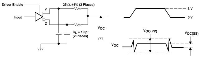
NOTE A: All input pulses are supplied by a generator having the following characteristics:  $t_r$  or  $t_f \le 1$  ns, pulse repetition rate (PRR) = 50 Mpps, pulse width = 10 ± 0.2 ns . C<sub>L</sub> includes instrumentation and fixture capacitance within 0,06 mm of the D.U.T. The measurement of V<sub>OC(PP)</sub> is made on test equipment with a –3 dB bandwidth of at least 300 MHz.
