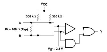
Figure 19. Open-Circuit Fail Safe of the LVDS Receiver
