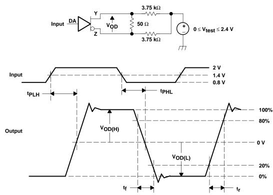
NOTE A: All input pulses are supplied by a generator having the following characteristics:  $t_f$  or  $t_f \le 1$  ns, pulse repetition rate (PRR) = 50 Mpps, pulse width = 10 ± 0.2 ns . C<sub>L</sub> includes instrumentation and fixture capacitance within 0,06 mm of the D.U.T.
