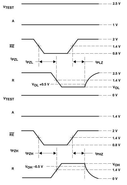
Figure 8. Enable/Disable Time Test Circuit and Waveforms
