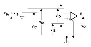
Figure 4. Receiver Voltage Definitions
