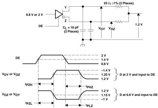
NOTE A: All input pulses are supplied by a generator having the following characteristics:  $t_r$  or  $t_f \le 1$  ns, pulse repetition rate (PRR) = 0.5 Mpps, pulse width = 500 ± 10 ns . CL includes instrumentation and fixture capacitance within 0,06 mm of the D.U.T.
