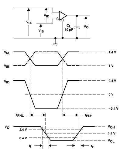
NOTE A: All input pulses are supplied by a generator having the following characteristics:  $t_r$  or  $t_f \le 1$  ns, pulse repetition rate (PRR) = 50 Mpps, pulse width = 10 ± 0.2 ns. CL includes instrumentation and fixture capacitance within 0,06 mm of the D.U.T.
