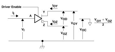
Figure 1. Driver Voltage and Current Definitions
