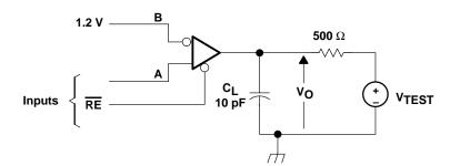
NOTE A: All input pulses are supplied by a generator having the following characteristics:  $t_r$  or  $t_f \le 1$  ns, pulse repetition rate (PRR) = 0.5 Mpps, pulse width = 500 ± 10 ns. C<sub>L</sub> includes instrumentation and fixture capacitance within 0,06 mm of the D.U.T.
