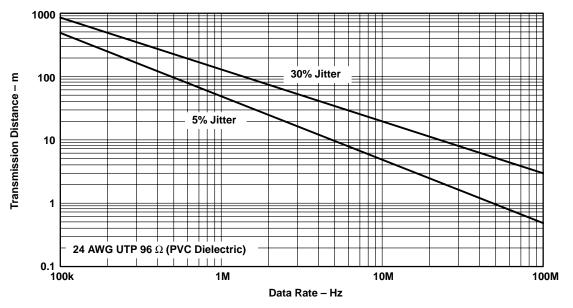
Figure 18. Data Transmission Distance Versus Rate
