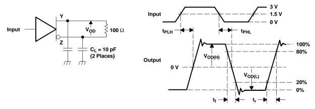
NOTE: All input pulses are supplied by a generator having the following characteristics:  $t_r$  or  $t_f \le 1$  ns, pulse repetition rate (PRR) = 50 Mpps, pulse width = 10 ±0.2 ns.  $C_L$  includes instrumentation and fixture capacitance within 0,06 mm of the DUT.
