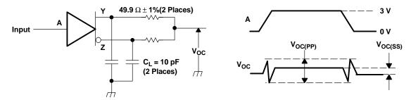
NOTE: All input pulses are supplied by a generator having the following characteristics: t<sub>r</sub> or t<sub>f</sub> ≤ 1 ns, pulse repetition rate (PRR) = 0.5 Mpps, pulse width = 500 ±10 ns. C<sub>L</sub> includes instrumentation and fixture capacitance within 0,06 mm of the DUT. The measurement of V<sub>OC(PP)</sub> is made on test equipment with a –3 dB bandwidth of at least 300 MHz.
