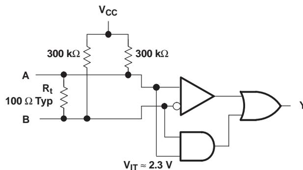
**Figure 23. Open-Circuit Fail Safe of the LVDS Receiver**
