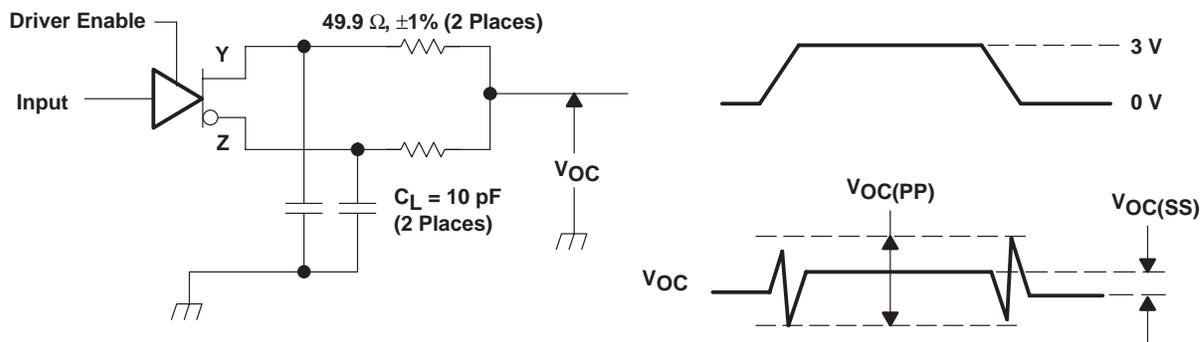
NOTE A: All input pulses are supplied by a generator having the following characteristics:  $t_r$  or  $t_f \leq 1$  ns, pulse repetition rate (PRR) = 50 Mpps, pulse width =  $10 \pm 0.2$  ns.  $C_L$  includes instrumentation and fixture capacitance within 0,06 mm of the D.U.T. The measurement of  $V_{OC(PP)}$  is made on test equipment with a  $-3$  dB bandwidth of at least 300 MHz.
