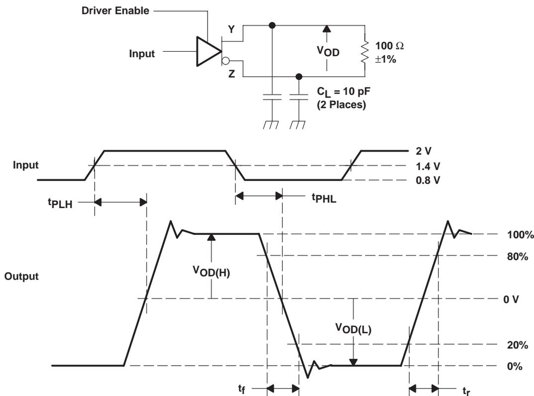
NOTE A: All input pulses are supplied by a generator having the following characteristics:  $t_r$  or  $t_f \leq 1$  ns, pulse repetition rate (PRR) = 50 Mpps, pulse width =  $10 \pm 0.2$  ns.  $C_L$  includes instrumentation and fixture capacitance within 0,06 mm of the D.U.T.
