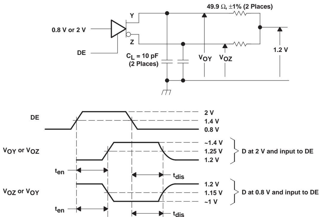
NOTE A: All input pulses are supplied by a generator having the following characteristics:  $t_r$  or  $t_f \leq 1$  ns, pulse repetition rate (PRR) = 0.5 Mpps, pulse width =  $500 \pm 10$  ns.  $C_L$  includes instrumentation and fixture capacitance within 0,06 mm of the D.U.T.
