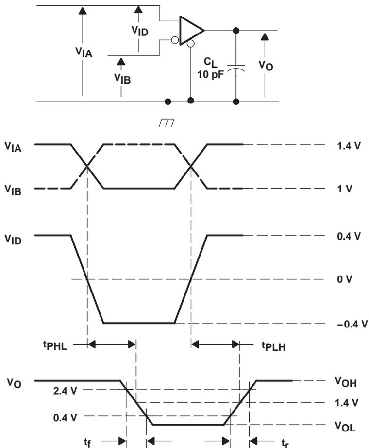
NOTE A: All input pulses are supplied by a generator having the following characteristics:  $t_r$  or  $t_f \leq 1$  ns, pulse repetition rate (PRR) = 50 Mpps, pulse width =  $10 \pm 0.2$  ns.  $C_L$  includes instrumentation and fixture capacitance within 0,06 m of the D.U.T.
