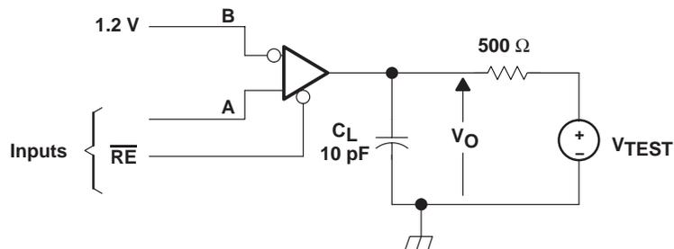
NOTE A: All input pulses are supplied by a generator having the following characteristics:  $t_r$  or  $t_f \leq 1$  ns, pulse repetition rate (PRR) = 0.5 Mpps, pulse width =  $500 \pm 10$  ns.  $C_L$  includes instrumentation and fixture capacitance within 0,06 m of the D.U.T.
