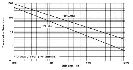
Figure 22. Data Transmission Distance Versus Rate
