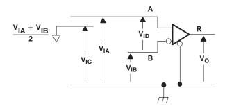
Figure 5. Receiver Voltage Definitions
