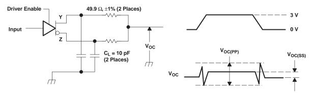
A. All input pulses are supplied by a generator having the following characteristics:  $t_r$  or  $t_f \le 1$  ns, pulse repetition rate (PRR) = 50 Mpps, pulse width = 10 ± 0.2 ns. C<sub>L</sub> includes instrumentation and fixture capacitance within 0,06 mm of the D.U.T. The measurement of V<sub>OC(PP)</sub> is made on test equipment with a –3-dB bandwidth of at least 300 MHz.
