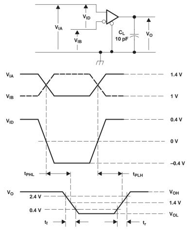
A. All input pulses are supplied by a generator having the following characteristics:  $t_r$  or  $t_f \le 1$  ns, pulse repetition rate (PRR) = 50 Mpps, pulse width = 10 ± 0.2 ns. C<sub>L</sub> includes instrumentation and fixture capacitance within 0,06 m of the D.U.T.
