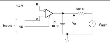
A. All input pulses are supplied by a generator having the following characteristics:  $t_r$  or  $t_f \le 1$  ns, pulse repetition rate (PRR) = 0.5 Mpps, pulse width = 500 ± 10 ns. C<sub>L</sub> includes instrumentation and fixture capacitance within 0,06 m of the D.U.T.
