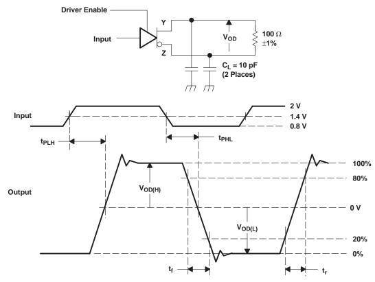
A. All input pulses are supplied by a generator having the following characteristics:  $t_r$  or  $t_f \le 1$  ns, pulse repetition rate (PRR) = 50 Mpps, pulse width = 10 ± 0.2 ns. C<sub>L</sub> includes instrumentation and fixture capacitance within 0,06 mm of the D.U.T.
