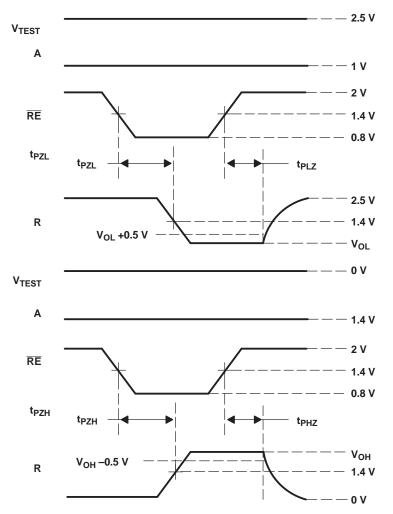
Figure 7. Enable/Disable Time Test Circuit and Waveforms
