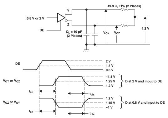
A. All input pulses are supplied by a generator having the following characteristics:  $t_r$  or  $t_f \le 1$  ns, pulse repetition rate (PRR) = 0.5 Mpps, pulse width = 500 ± 10 ns.  $C_L$  includes instrumentation and fixture capacitance within 0,06 mm of the D.U.T.
