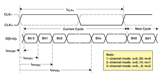
Figure 13. t<sub>SK(0)</sub> SubLVDS Output Pulse Position Measurement
