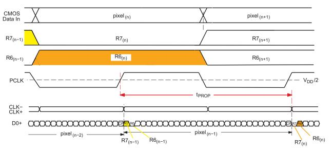
Figure 11. t<sub>pd(L)</sub> Propagation Delay Input to Output (LS0 = LS1 = 0; CPOL = 0)
