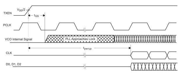
Figure 14. Transmitter Behavior While Approaching Sync
