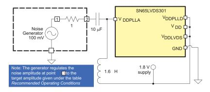
Figure 12. Power Supply Noise Test Set-Up
