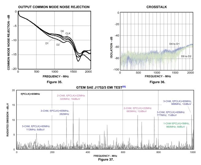
A. Figure 37 shows a superimposed image of three EMI measurements with the device operating at f(PCLK) = 5 MHz, f(PCLK) = 22 MHz, and f(PCLK) = 65 MHz. This excellent EMI performance meets the system requirements of dense, mobile designs with a noise floor of ~2 dBμV (-105 dBm) and all spurs being smaller than 16 dBμV (-101 dBm). The test was performed in compliance with the SAE J1752/3 EMI test guidelines.
