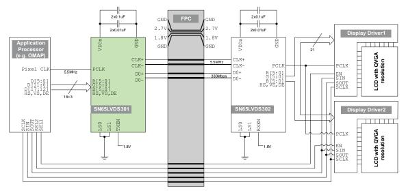
Figure 39. Example Dual-QVGA Display Application
