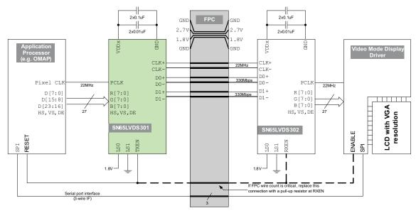
Figure 38. Typical VGA Display Application
