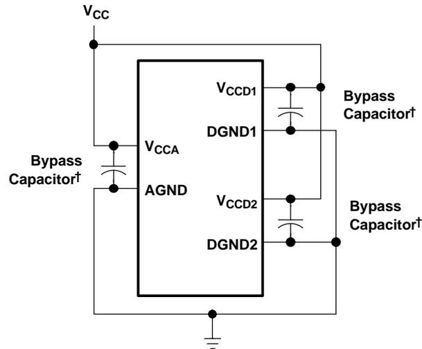
† Bypass capacitors used for data sheet electrical testing were low ESR ceramic, surface mount, 0.01  $\mu\text{F} \pm 10\%$ . For a more accurate determination of these values refer to the application note, *The Bypass Capacitor in High-Speed Environments*, literature number SCBA007A.
