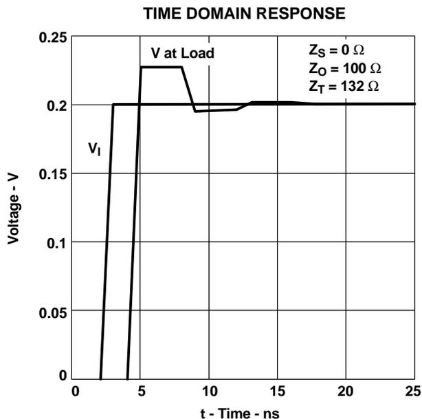
Figure 14. Low-Source Impedance
