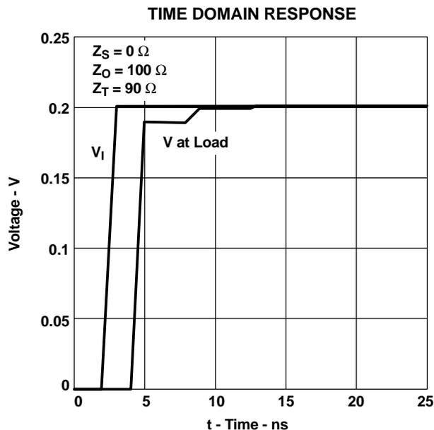
Figure 15. High-Source Impedance
