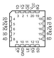
To ensure the high-impedance state during power up or power down,  $\overline{\text{OE}}$  should be tied to V<sub>CC</sub> through a pullup resistor; the minimum value of the resistor is determined by the current-sinking capability of the driver.
