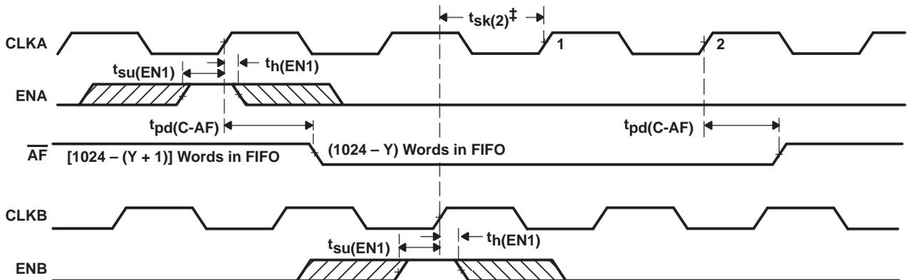
‡  $t_{sk(2)}$  is the minimum time between a rising CLKA edge and a rising CLKB edge for  $\overline{AF}$  to transition high in the next CLKA cycle. If the time between the rising CLKB edge and rising CLKA edge is less than  $t_{sk(2)}$ ,  $\overline{AF}$  can transition high one CLKA cycle later than shown.
