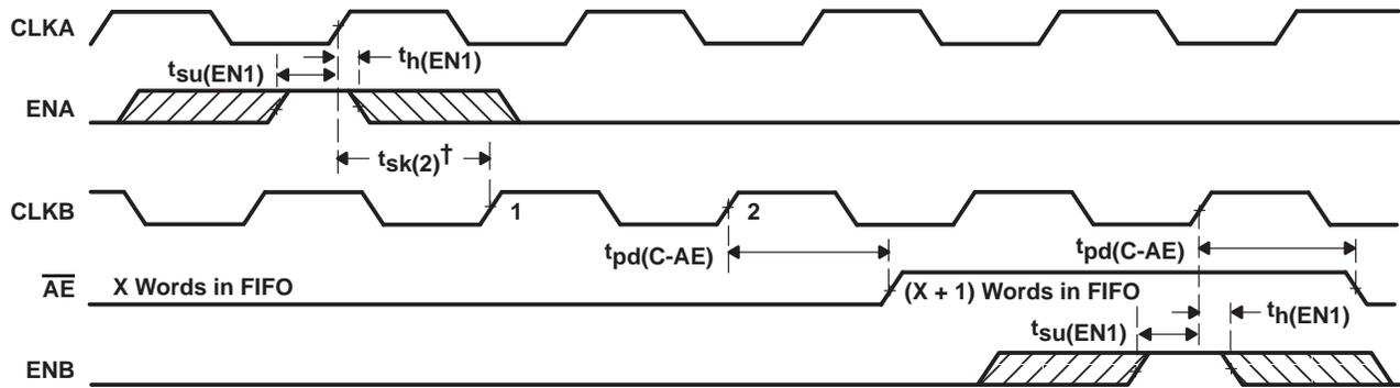
†  $t_{sk(2)}$  is the minimum time between a rising CLKA edge and a rising CLKB edge for  $\overline{AE}$  to transition high in the next CLKB cycle. If the time between the rising CLKA edge and rising CLKB edge is less than  $t_{sk(2)}$ ,  $\overline{AE}$  can transition high one CLKB cycle later than shown.
