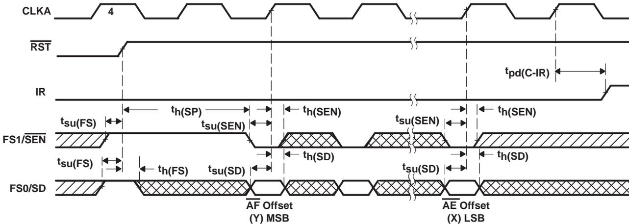
NOTE A: It is not necessary to program offset register bits on consecutive clock cycles. FIFO write attempts are ignored until IR is set high.
