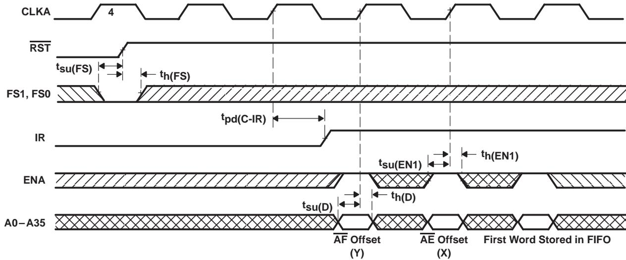
NOTE A:  $\overline{CSA} = L$ ,  $W/\overline{RA} = H$ ,  $MBA = L$ . It is not necessary to program offset register on consecutive clock cycles.
