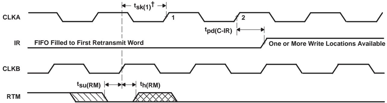
$^\dagger t_{sk(1)}$  is the minimum time between a rising CLKB edge and a rising CLKA edge for IR to transition high in the next CLKA cycle. If the time between the rising CLKB edge and rising CLKA edge is less than  $t_{sk(1)}$ , IR can transition high one CLKA cycle later than shown.
