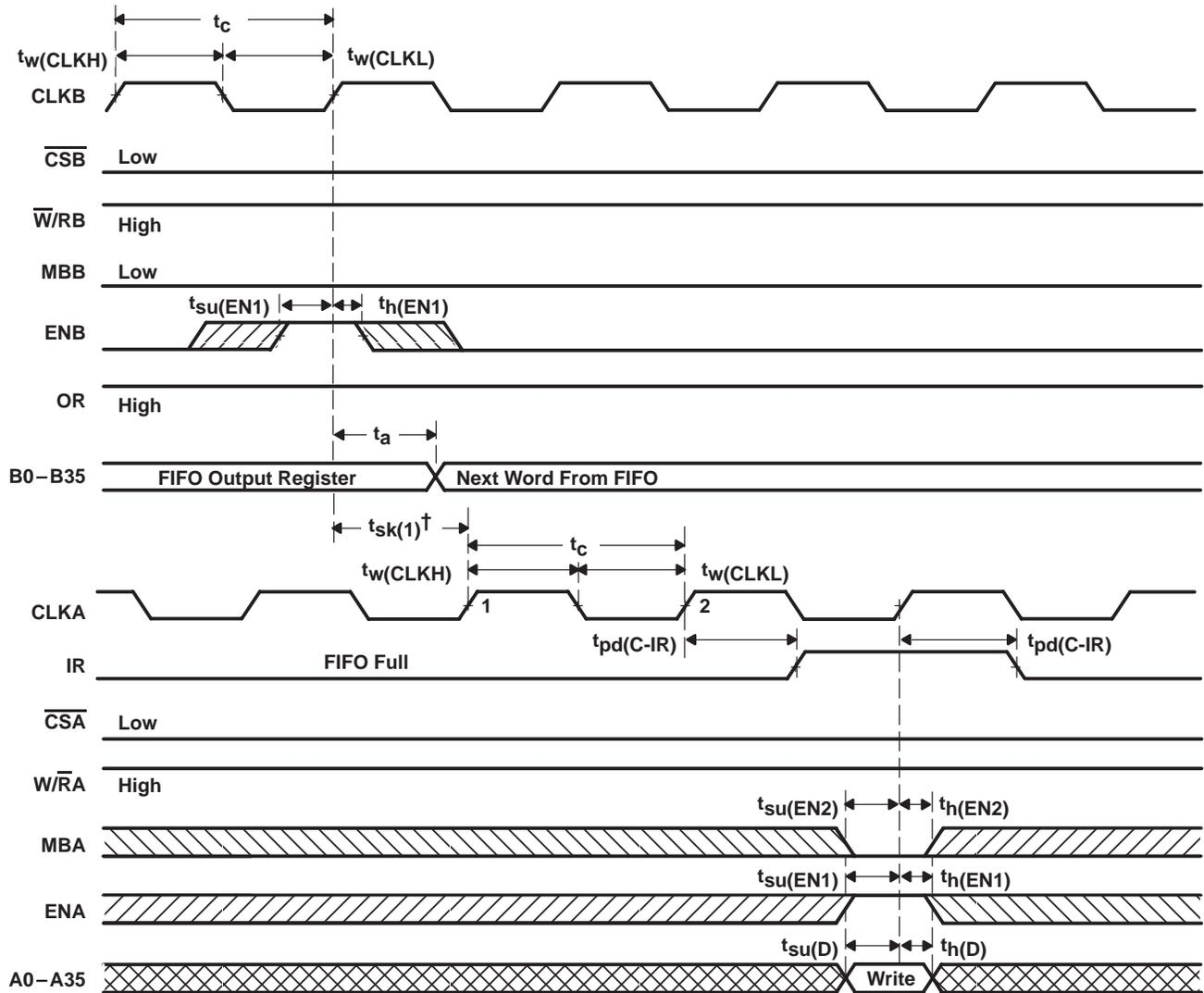
$\dagger t_{sk(1)}$  is the minimum time between a rising CLKB edge and a rising CLKA edge for IR to transition high in the next CLKA cycle. If the time between the rising CLKB edge and rising CLKA edge is less than  $t_{sk(1)}$ , IR can transition high one CLKA cycle later than shown.
