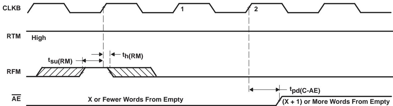
NOTE A: X is the value loaded in the  $\overline{AE}$  flag offset register.
