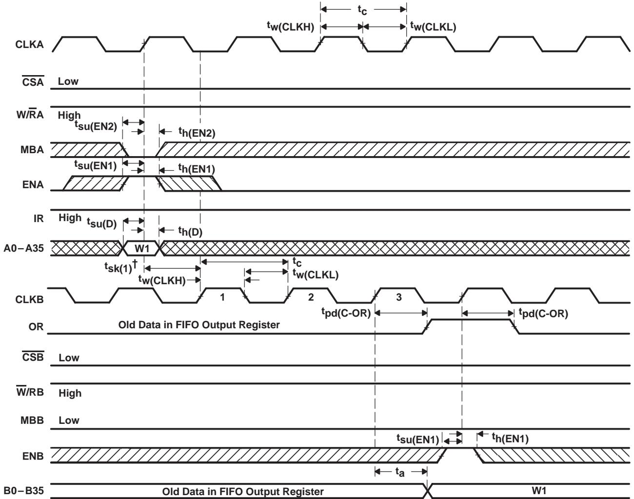
$^\dagger t_{sk}(1)$  is the minimum time between a rising CLKA edge and a rising CLKB edge for OR to transition high and to clock the next word to the FIFO output register in three CLKB cycles. If the time between the rising CLKA edge and rising CLKB edge is less than  $t_{sk}(1)$ , the transition of OR high and the first word load to the output register can occur one CLKB cycle later than shown.
