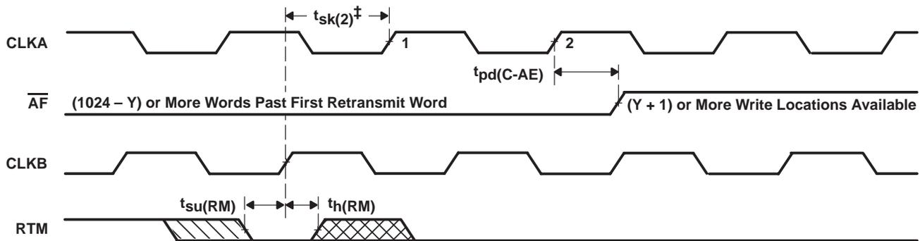
$^\ddagger t_{sk(2)}$  is the minimum time between a rising CLKB edge and a rising CLKA edge for  $\overline{AF}$  to transition high in the next CLKA cycle. If the time between the rising CLKB edge and rising CLKA edge is less than  $t_{sk(2)}$ ,  $\overline{AF}$  can transition high one CLKA cycle later than shown.
