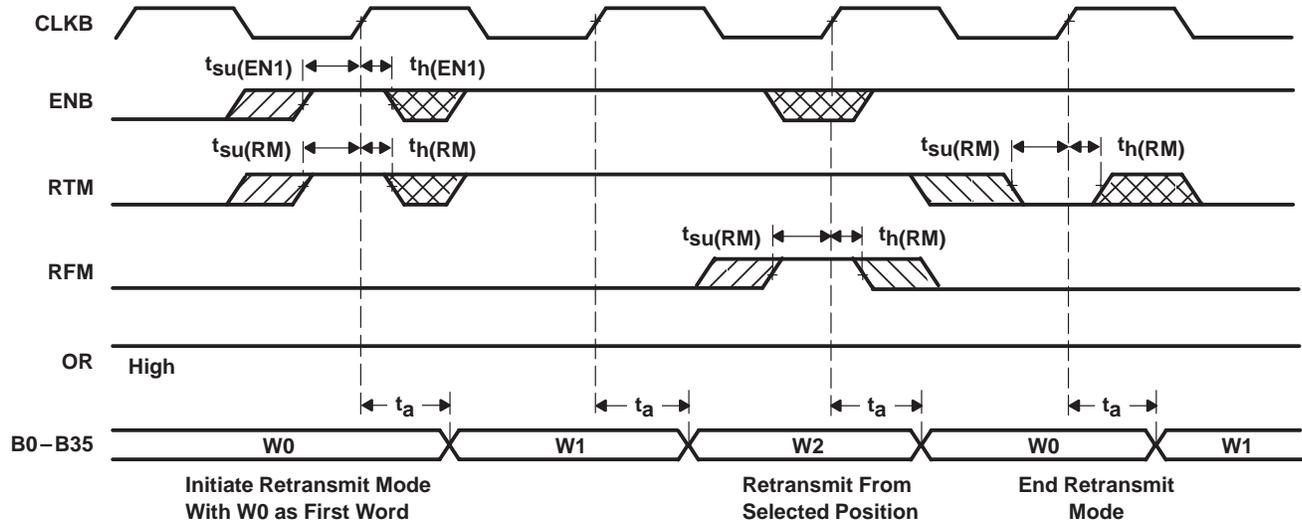
NOTE A:  $\overline{CSB} = L$ ,  $\overline{WB/RB} = H$ ,  $MBB = L$ . No input enables other than RTM and RFM are needed to control retransmit mode or begin a retransmit. Other enables are shown only to relate retransmit operations to the FIFO output register.
