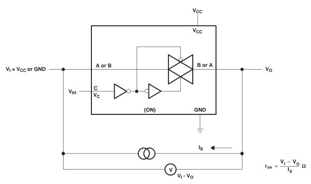
Figure 1. On-State Resistance Test Circuit
