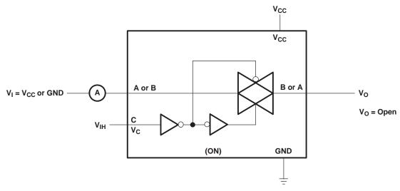
Figure 3. On-State Leakage-Current Test Circuit
