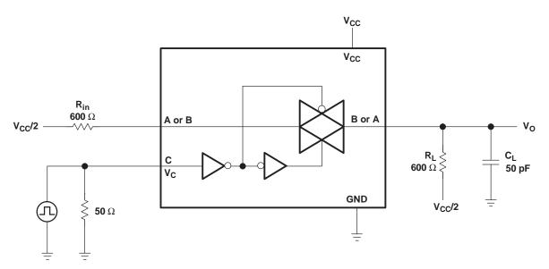
Figure 6. Crosstalk (Control Input – Switch Output)
