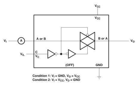
Figure 2. Off-State Switch Leakage-Current Test Circuit
