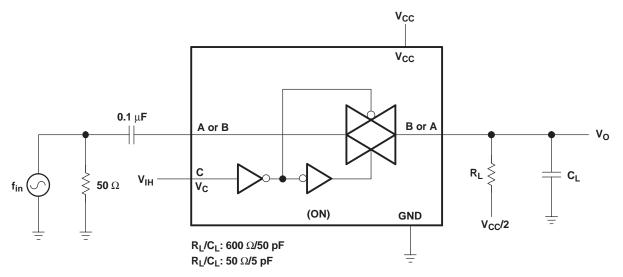
Figure 5. Frequency Response (Switch ON)
