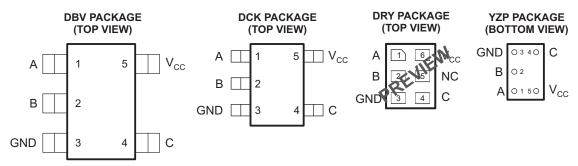
See mechanical drawings for dimensions. NC- No internal connection
