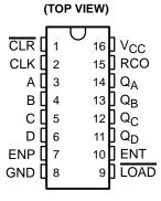
so instructed by the count-enable (ENP, ENT) inputs and internal gating. This mode of operation eliminates the output counting spikes that are normally associated with asynchronous (ripple-clock) counters. However, counting spikes can occur on the ripple-carry (RCO) output. A buffered clock (CLK) input triggers the four flip-flops on the rising (positive-going) edge of CLK.
