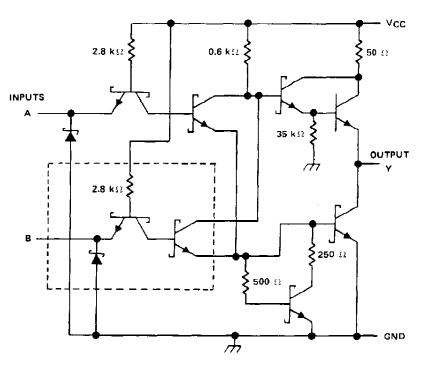
Resistor values shown are nominal. The portion of the schematic within the deshed-line is repeated for each additional input.
