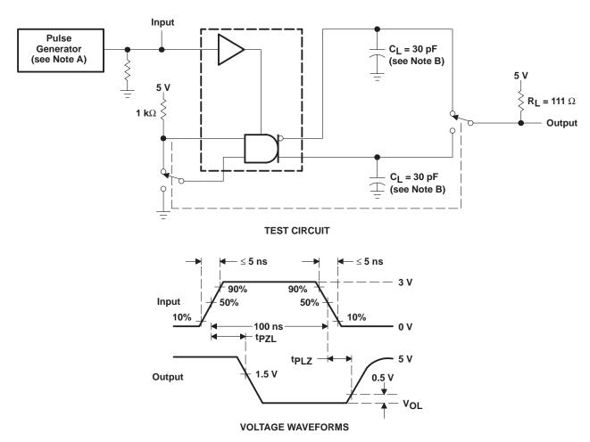
NOTES: A. The pulse generators have the following characteristics:  $Z_0$  = 50  $\Omega$ , PRR  $\leq$  500 kHz.
