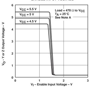
NOTE A: The A input is connected to GND during the testing of the Y outputs and to V<sub>CC</sub> during the testing of the Z outputs.
