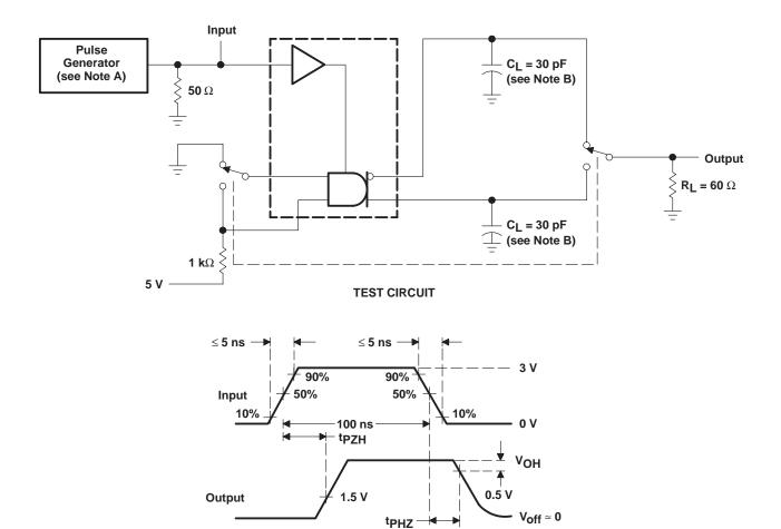
NOTES: A. The pulse generator has the following characteristics: Z<sub>O</sub> = 50  $\Omega$ , PRR  $\leq$  500 kHz.
