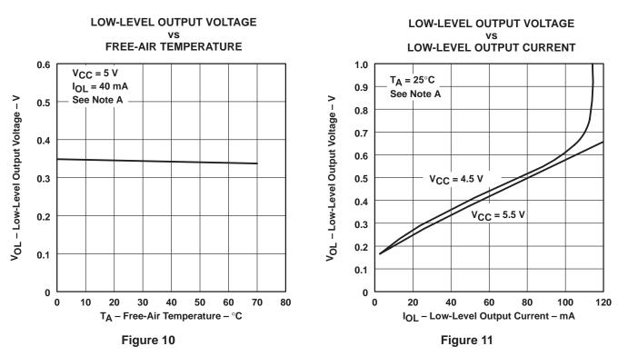
NOTE A: The A input is connected to GND during the testing of the Y outputs and to V<sub>CC</sub> during the testing of the Z outputs.
