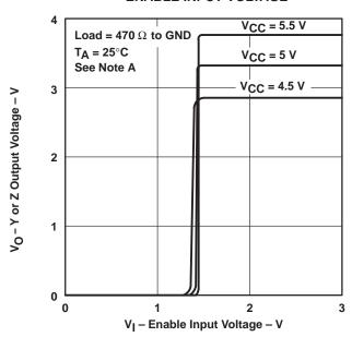
NOTE A: The A input is connected to V<sub>CC</sub> during the testing of the Y outputs and to ground during testing of the Z outputs.
