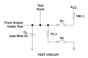
NOTES: A. When measuring propagation delay times and skew, switches S1 and S2 are open.
