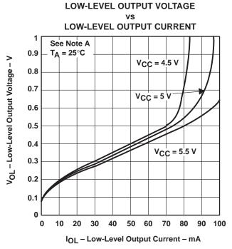
NOTE A: The A input is connected to GND during the testing of the Y outputs and to  $V_{\hbox{CC}}$  during the testing of the Z outputs.
