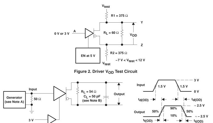
NOTES: A. The input pulse is supplied by a generator having the following characteristics: PRR  $\leq$  1 MHz, duty cycle  $\leq$  50%, t<sub>f</sub>  $\leq$  5 ns, t<sub>f</sub>  $\leq$  5 ns, Z<sub>O</sub> = 50  $\Omega$ .
