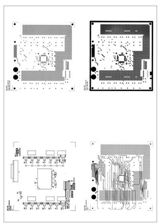
Figure 14a. Evaluation Board — Top Layers
