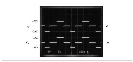
Figure 3. Charge Pump Waveforms
