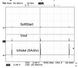
Figure 8. Output Load Short Circuit
