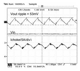
Figure 17. Output Ripple: 8A Load
