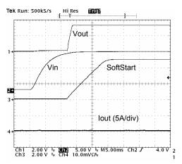
Figure 5. Start-Up Response: No Load
