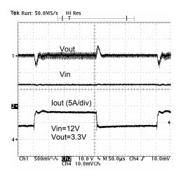
Figure 3. Load Step Response: 4->8A
