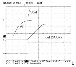
Figure 7. Start-Up Response: 8A Load
