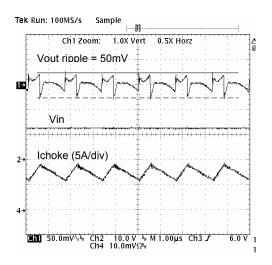
Figure 9. Output Ripple: No Load
