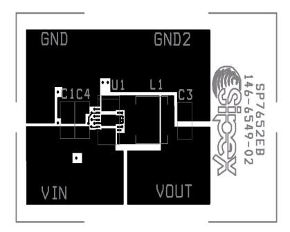
Figure 26. SP7652EB PC Layout Top Side
