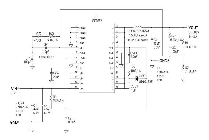
Figure 13. SP7652EU Configures for Vin = 5V, Vout = 3.3V at 0-8A Output Load Current
