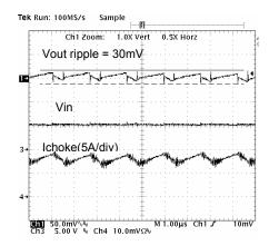
Figure 21. Output Ripple: No Load
