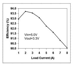
Figure 23. Efficiency vs Load
