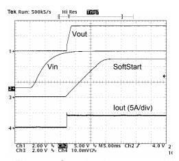
Figure 6. Start-Up Response: 4A Load
