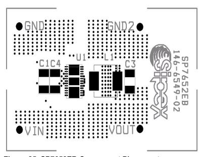
Figure 25. SP7652EB Component Placement
