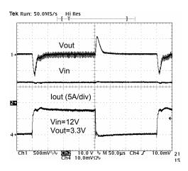
Figure 4. Load Step Response: 0->8A
