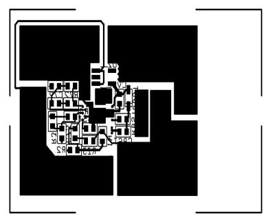
Figure 29. SP7652EB PC Layout Bottom Side
