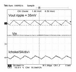
Figure 16. Output Ripple: No Load
