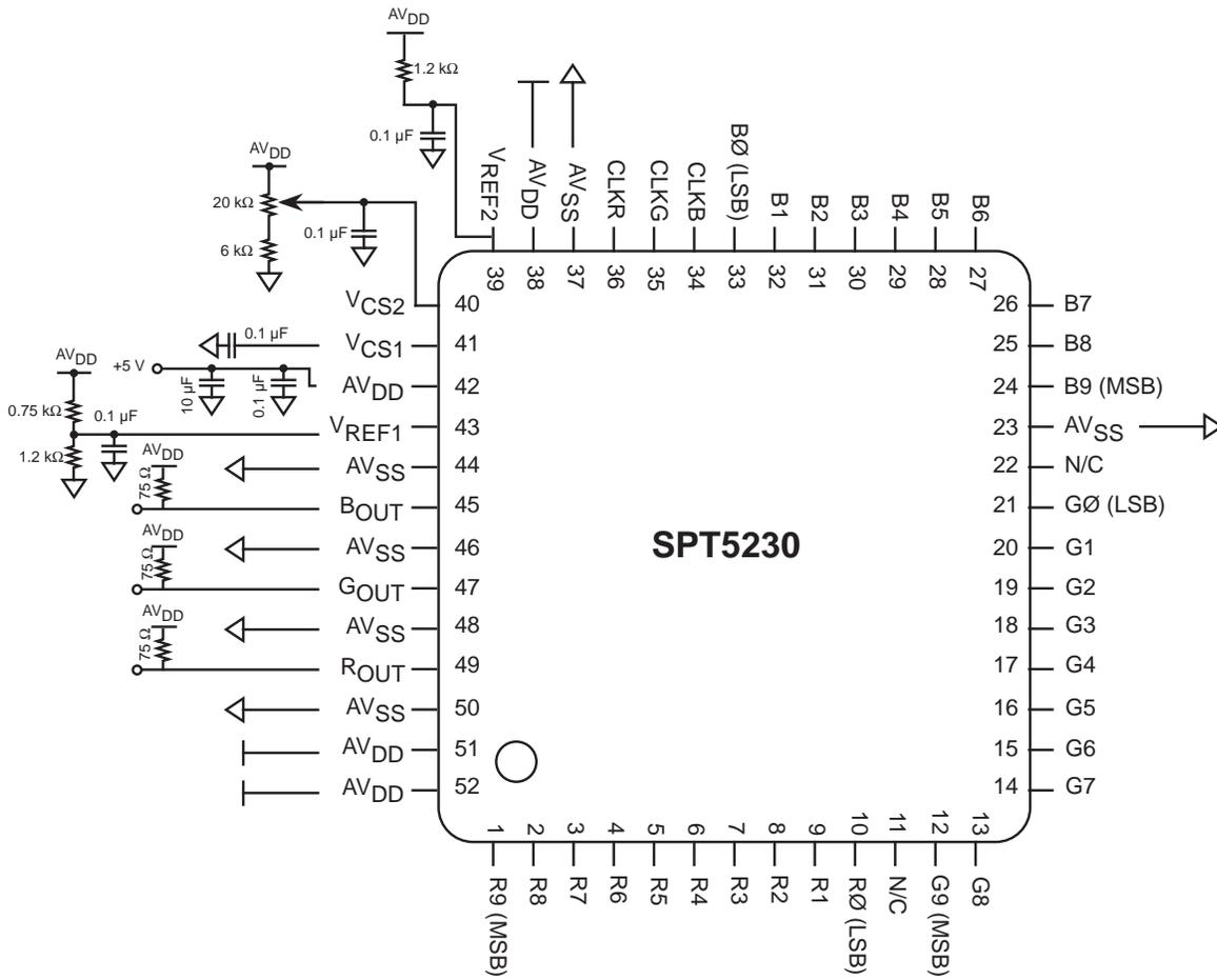
Figure 5 – Recommended Output Level Shifting Circuit
