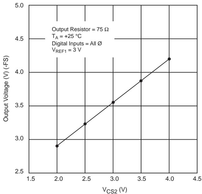
NOTE: For Digital Inputs = All 1, Output Voltage = +4.998047 V.
