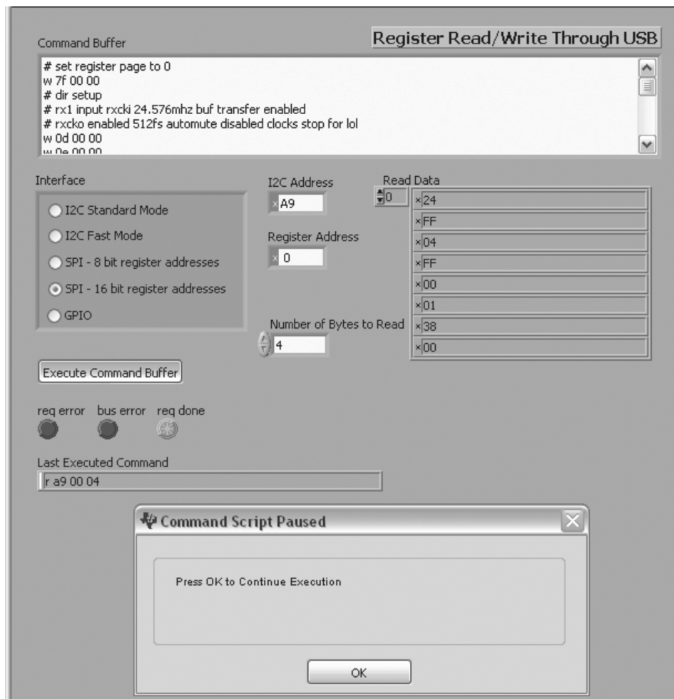
Figure 5. Example of a Readback Display and Break Message in the USB Serial Commander Application
