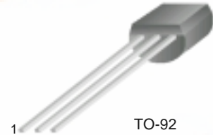
TO-92 1. Emitter 2. Base 3. Collector
