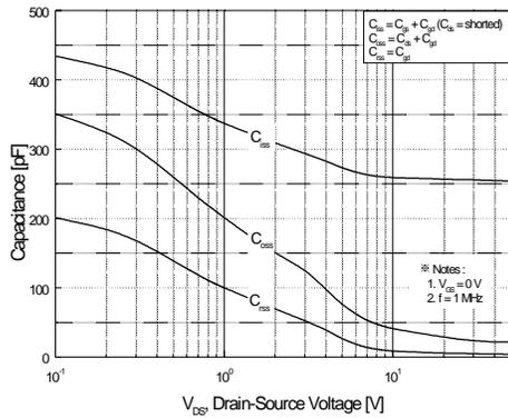
Figure 5. Capacitance Characteristics
