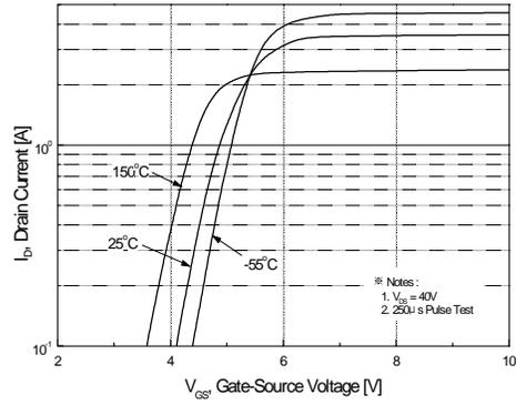
Figure 2. Transfer Characteristics
