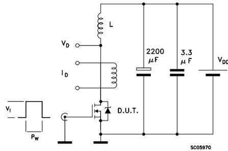
Figure 17. Unclamped Inductive Waveform
