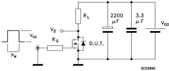
Figure 15. Gate Charge Test Circuit
