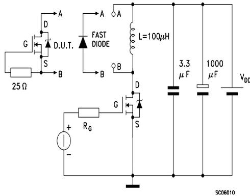
Figure 18. Unclamped Inductive Load Test Circuit
