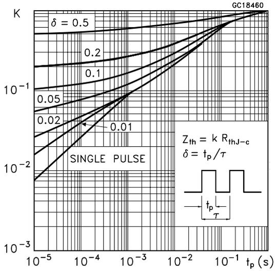
**Thermal Impedance for ISOWATT218**
