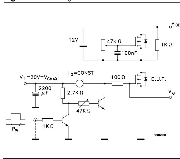
**Fig. 5:** Test Circuit For Inductive Load Switching And Diode Recovery Times
