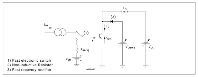
Figure 2: Resistive Load Switching Test Circuit.
