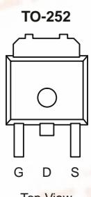
Drain Connected to Tab
