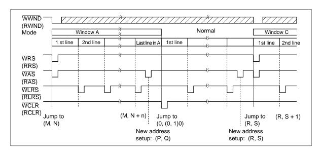
Case 4: Switching from Window A Scan to Window B Scan to Window C Scan
