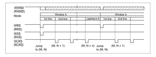
Case 3: Switching from Window A Scan to Normal Scan to Window C Scan
